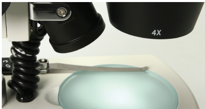
Close-up of stage plate from 591815 Wolfe Student Stereomicroscope, 20× and 40× Magnification
